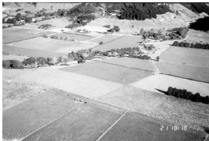
FIGURE C4.2.1(C) TYPICAL EXAMPLE OF TERRAIN CATEGORY 2 Excerpt from AS/NZS 1170.2 Supplement 1:2002
