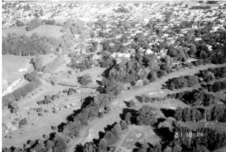
FIGURE C4.2.1(D) TYPICAL EXAMPLE OF TERRAIN CATEGORY 3 Excerpt from AS/NZS 1170.2 Supplement 1:2002
