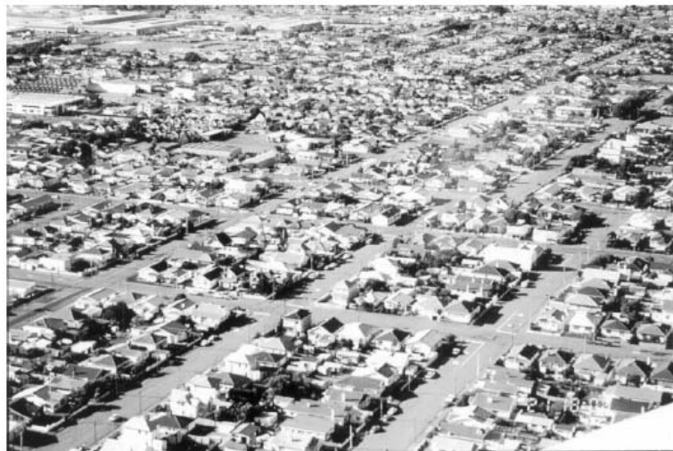
FIGURE C4.2.1(E) TYPICAL EXAMPLE OF TERRAIN CATEGORY 3 Excerpt from AS/NZS 1170.2 Supplement 1:2002
