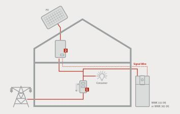
SG Ready implementation of connecting the STIEBEL ELTRON WWK hot water heat pump allows for a higher water temperature and more "free" hot water. A signal wire is connected from the solar PV inverter \* to the WWK activating a higher secondary water temperature set point.
